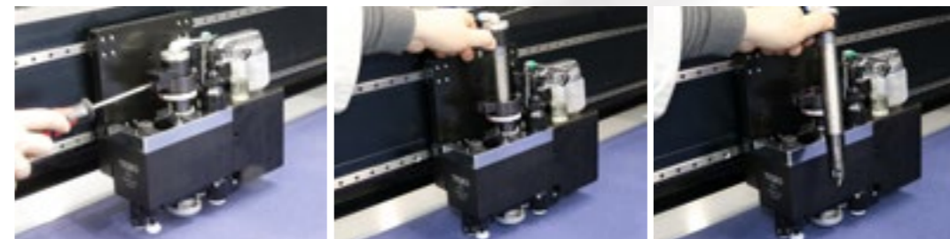
Changing blade or oscillating knife in less than 45 seconds .
