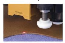
Thanks to the **3D** vision, ARGHON is constantly capable of measuring the wear of the cutting carpet and the hide thickness, detecting variations in height.
