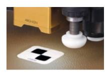
ARGHON recognizes details size less than **0.1 mm**. It enables a better recognition of **ROT** (Reference Optical Tag) for automatic hide re-positioning.
