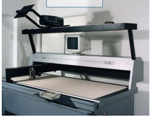
THE FIRST AUTOMATIC CUTTER WITH AN OSCILLATING KNIFE FOR LEATHER
